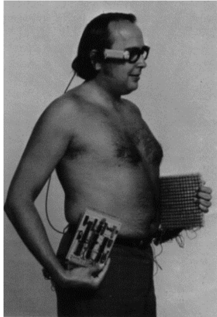
Figure 12-1. A later, portable, version of Bach y Rita's Tactile Visual Substitution System, with an array of vibrators to be worn on the abdomen, and with portable electronics and a camera mounted on a pair of spectacles. Using such a system, a person is able to navigate around the room within seconds of putting on the device, and is able to recognize simple objects with minimal training by "scanning" them using head movements.
