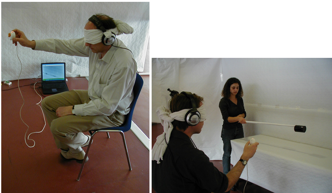
Figure 12-2. Left: Sensory substitution researcher and philosopher Charles Lenay trying out Peter Meijer's The vOICe in my laboratory in Paris. Blindfolded, he is holding a webcam connected to a laptop which is converting the image into a "soundscape" that is scanned twice per second, and which he is listening to through headphones.
