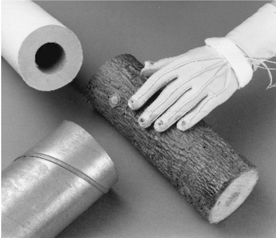
Figure 12-3. A tactile glove equipped with miniature condenser microphones on the fingertips. Transmitted to earphones worn by the user, the sound from these can be used to allow an observer to distinguish between different textures, here wood, paper and metal 232 .
